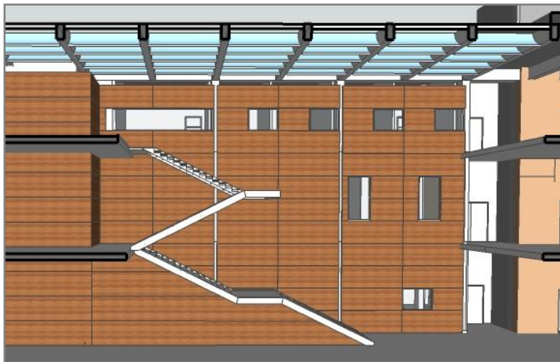
Straight then Switchback Stair
