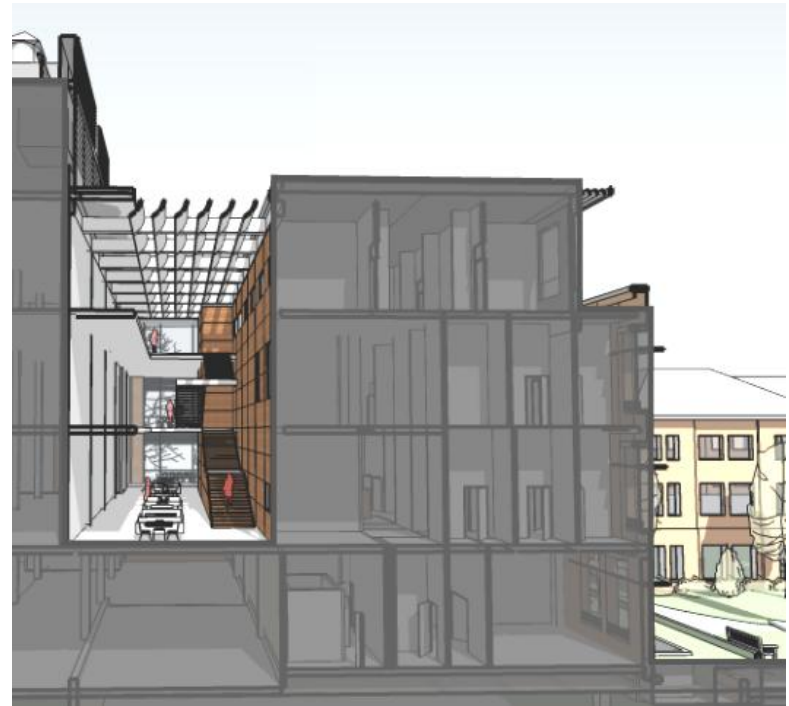
Atrium Starting at the Second Floor
